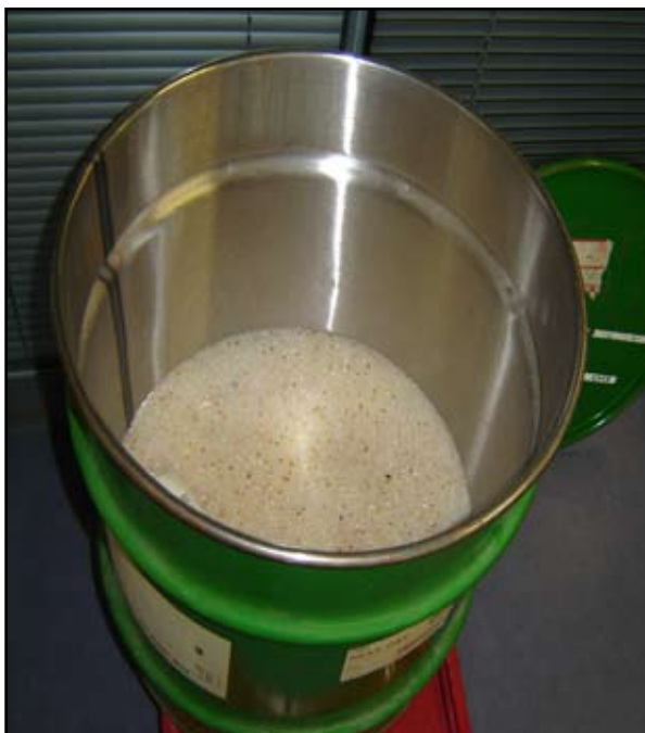
Figure 13 Silica gel drying bin. (© RBGK)
