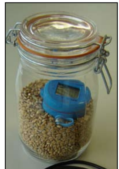
Figure 16 Datalogger recording eRH in a sealed container of seeds. (© RBGK)
