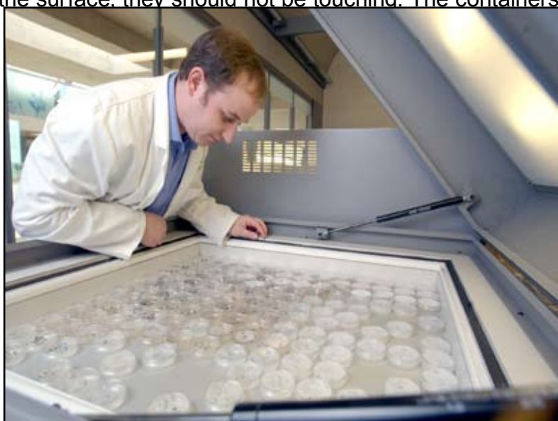
Figure 23 Incubator simulating day/night conditions. (© RBGK)
